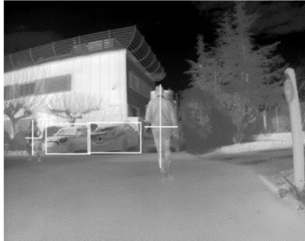
Figure 5: The Bertin Technologies CamSight AI is a low-SWaP camera performing real-time AI-based recognition and identification of targets—pedestrians and vehicles—in thermal imagery, with power consumption on the order of 4 W.
