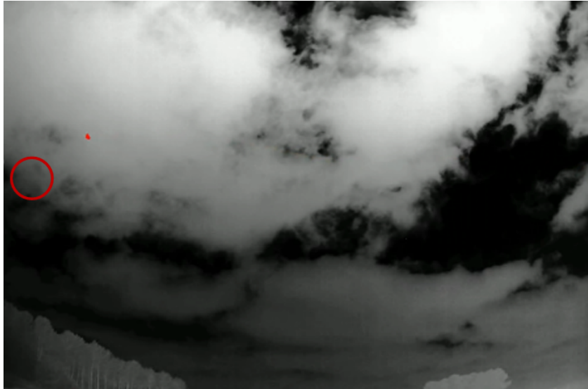
Figure 7: Bertin Technologies has developed a neural network for early detection of aerial drones, enabling real-time AI detection through the analysis of background-scene anomalies while remaining insensitive to moving distractors such as clouds.
