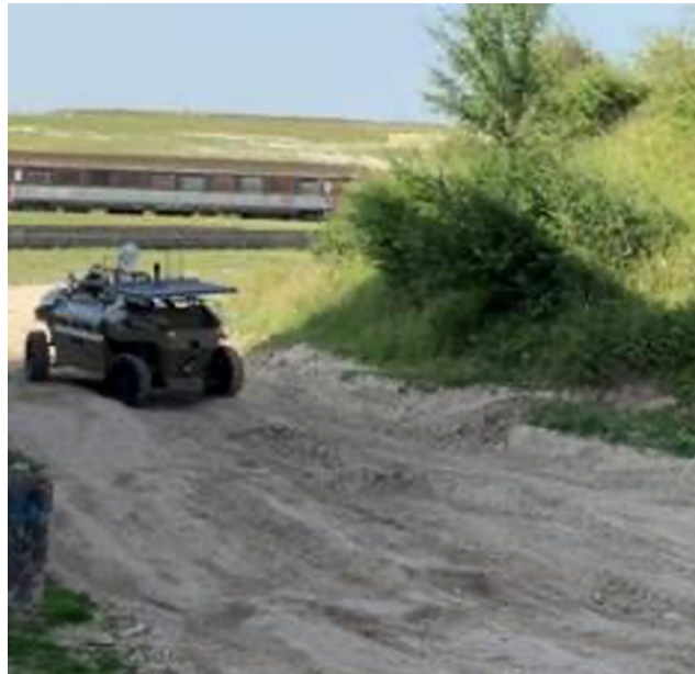
Figure 10: FURIOUS robotic vehicle after an obstacle-crossing phase in full autonomy during operational trials at CENZUB.
