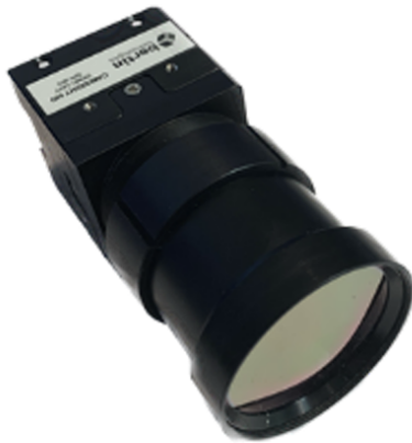
Figure 5: The Bertin Technologies CamSight AI is a low-SWaP camera performing real-time AI-based recognition and identification of targets—pedestrians and vehicles—in thermal imagery, with power consumption on the order of 4 W.
