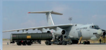
Refueler 8000 USG 300 GPM - Large display Underwing - Overwing Autoadaptive system
