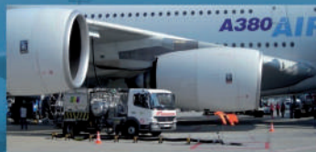
Dispenser 900 GPM Paris Airport
